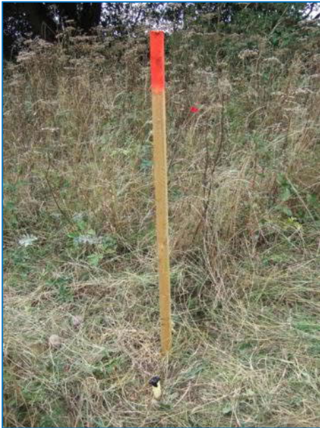
Photo 18. Dipwell T2-D at the SE SSSI unit.
